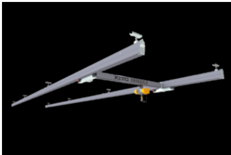
Single girder crane (steel bridge and track)
