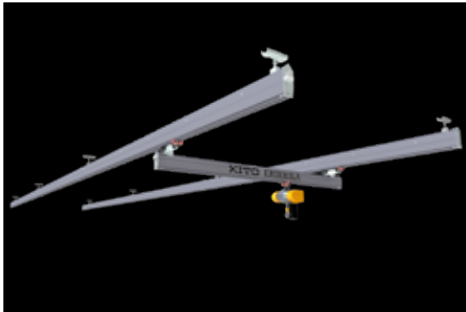
Single girder crane (steel bridge and track)
